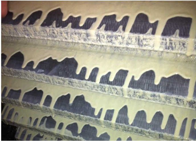
Lubrication film after 6 hours shutdown of a cement mill / spray application
