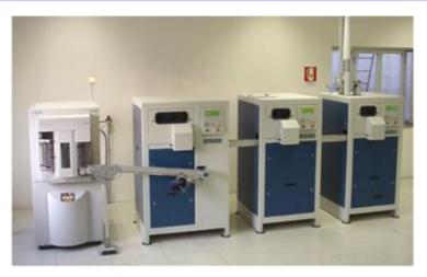
HR-LA, Mill & Press with XRF
