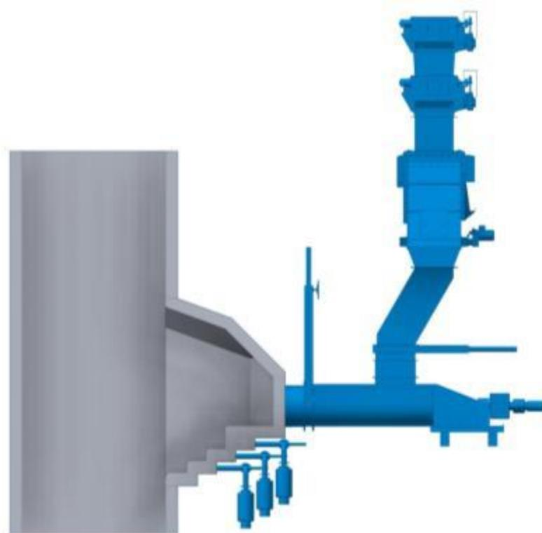
Fuel drying and pyrolysis in Prepol SC-S – char oxidation in calciner riser duct
