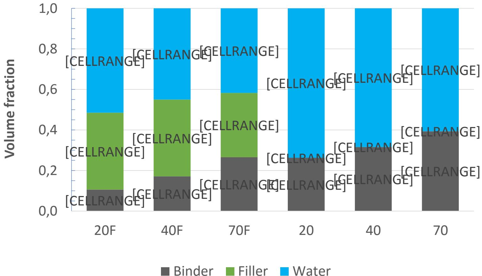
Data from Proske et al. Approach for eco-friendly concretes with reduced water and cement content. ICCS 2013. p288 .
