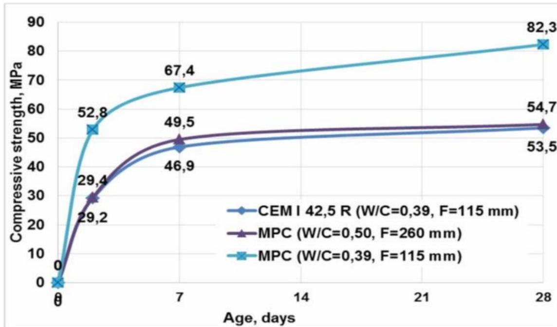
Figure 4 Compressive strength of portland cement CEM I and multimodal Portland cement (MPC)
