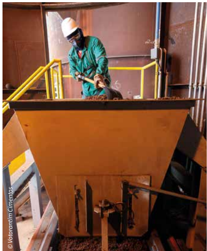
Top: co-processing of waste-derived fuel at Votorantim Cimentos Rio Branco do Sul plant in Brazil. Right: co-processing of açai seeds at the Primavera cement plant, Brazil
